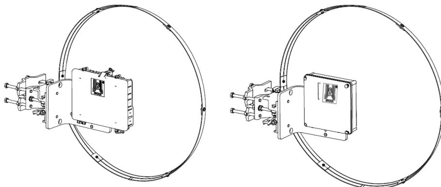
Accessories: outdoor plastic box JR – 200 or metal box JR – 250 Alu – right side mounting only, polarization 45° not possible
