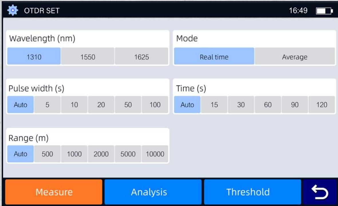
Acquisition parameters, such as range or duration, can be set manually or automatically. One-click testing is available for fiber cabling length and total loss, eliminating tedious operations.
