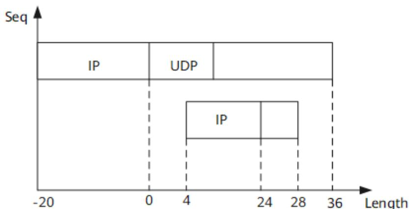
Teardrop attacks cause the system to restart or even crash. With defense against fragmentation attacks enabled, the device discards all fragments in a Teardrop attack.
