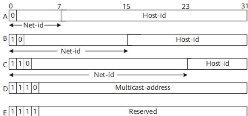
Most IP addresses in use belong to Class A, Class B, or Class C. Class D addresses are multicast addresses, and Class E addresses are reserved. The easiest way to determine the class of an IP address is to check the first bits in its network ID. The class fields of Class A, Class B, Class C, Class D, and Class E are binary numbers 0, 10, 110, 1110, and 1111, respectively.
