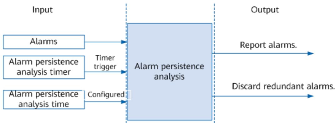
Alarm persistence analysis measures the duration after an alarm (a fault alarm or clear alarm) is generated. If the period defined for an alarm has elapsed but the alarm persists, a notification is sent. If an alarm is cleared within the defined period, the alarm is filtered out and no notification is sent. That is, if an alarm persists for a short time, it is filtered out and no notification is reported. Only stable fault information is displayed in the case of fault flapping.
