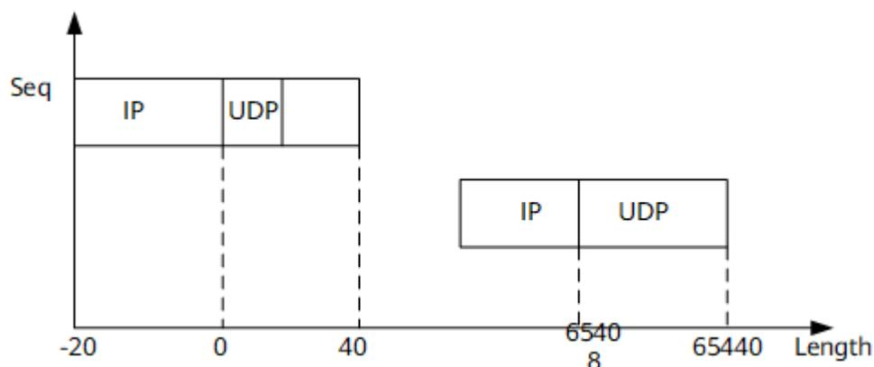
Rose attacks cause the system to restart or even crash. With defense against fragmentation attacks enabled, the device discards all fragments in a Rose attack.
