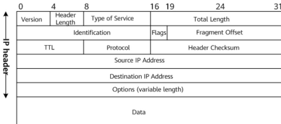
An IPv4 datagram consists of a header and a data field. The first 20 bytes in the header are mandatory for all IPv4 datagrams. The Options field following the 20 bytes has a variable length.
