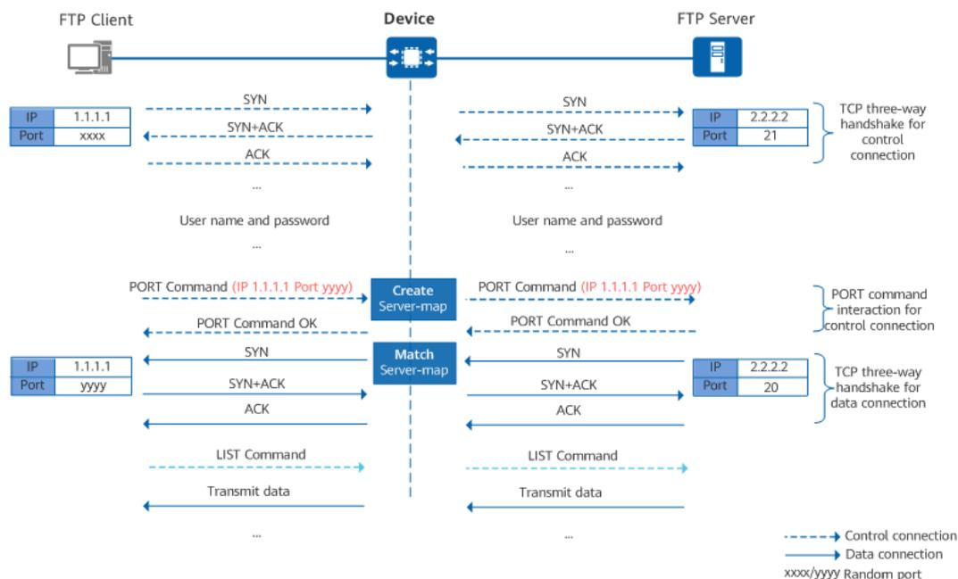
Port yyyy is the data port opened by the client to the server through the control channel. The data packet for the server (2.2.2.2) to proactively access port yyyy of the client (1.1.1.1) matches the server mapping entry and is permitted.
