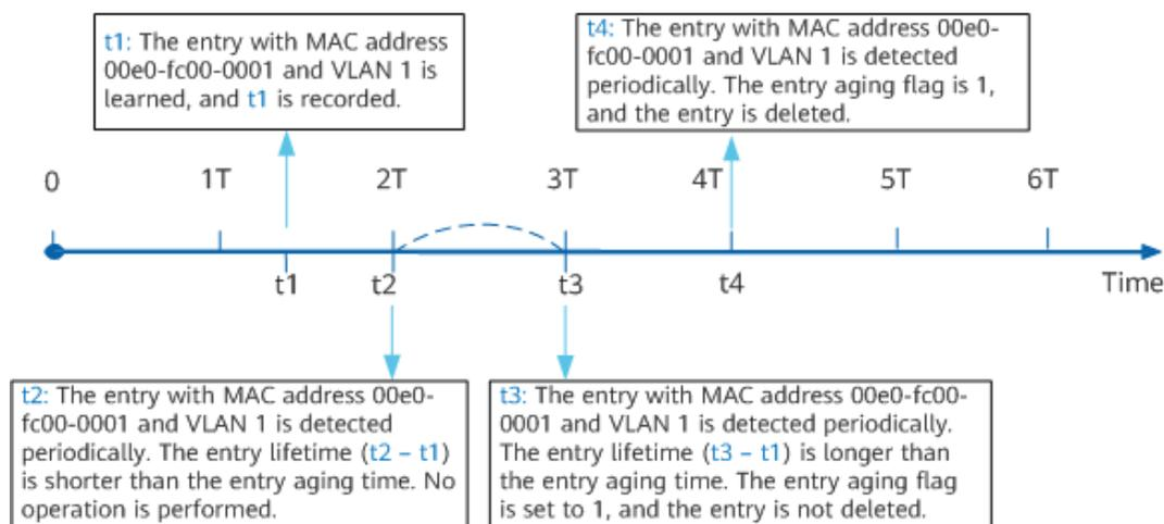
As shown in [Figure 5-3](#), the aging time of MAC address entries is set to 70 seconds in the following example.
