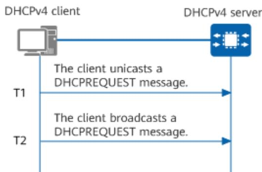
1. When the lease reaches 50% (T1) of its validity period, the DHCPv4 client unicasts a DHCPREQUEST message to the DHCPv4 server to request lease renewal. If the DHCPv4 client receives a DHCPACK message, the IPv4 address lease is successfully renewed (counted from 0). If the DHCPv4 client receives a DHCPNAK message, the DHCPv4 client must send a DHCPDISCOVER message to apply for a new IPv4 address.
