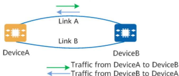
Symmetric load balancing ensures packet sequence but not bandwidth utilization.
