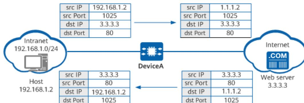
When a host on the intranet accesses the web server on the Internet, the source NAT process on DeviceA is as follows:
