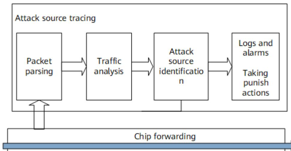
In this process, the device finds the attack source, triggers an alarm when detecting the packet rate exceeds the threshold, and takes punishment actions to protect the CPU.
