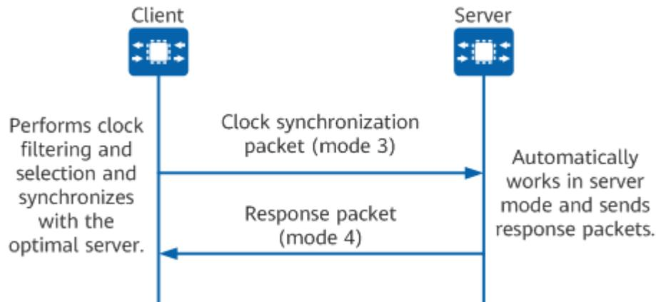
The packet exchange process in client/server mode is as follows:
