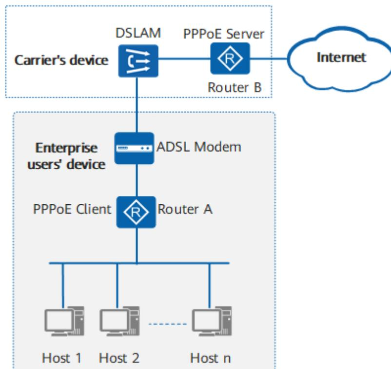
A device functions as a PPPoE server to dynamically allocate IP addresses to clients and provide multiple authentication methods. The PPPoE server is applicable to Ethernet networks connecting to the Internet, such as school campus networks and residential networks.
