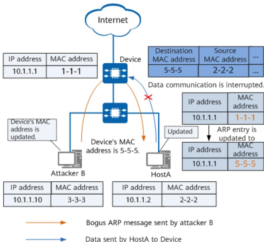
To prevent bogus gateway attacks, enable ARP gateway anti-collision on Device. In addition, you can enable gratuitous ARP message sending on Device so that Device can broadcast correct gratuitous ARP messages to all user hosts. In this manner, the gateway address mappings recorded by the attacked user hosts can be corrected.
