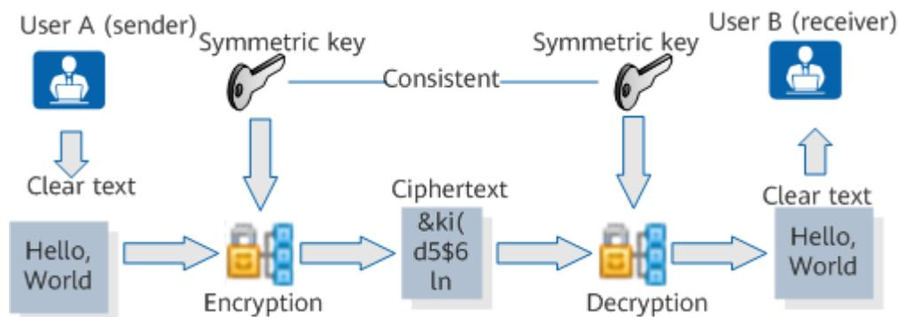
Users A and B have negotiated the symmetric key. The encryption and decryption process is as follows:
