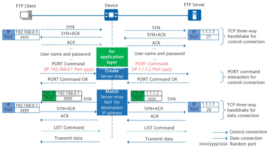
Before ALG is configured, the device translates only the IP address and port information in the packet header when performing source NAT. However, the IP address and port information carried in the packet payload remain unchanged. If the IP addresses and port numbers of both sides are different, FTP cannot work properly.
