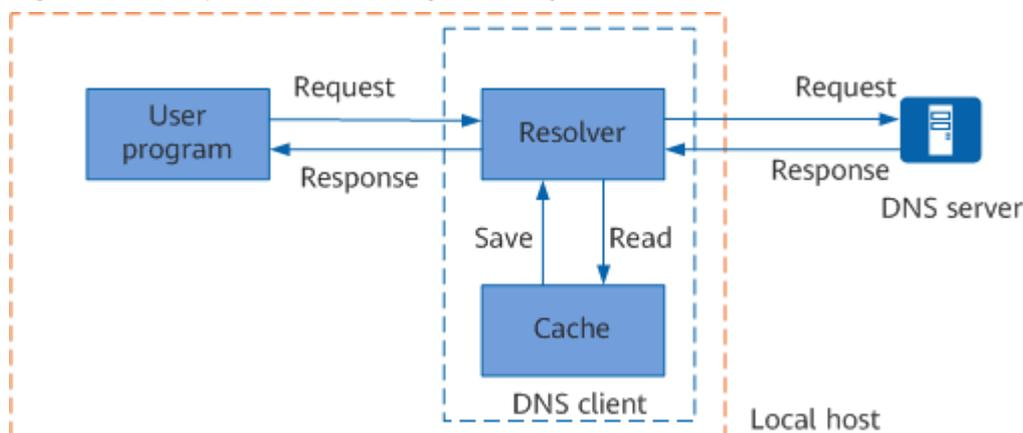
In [Figure 7-32](#), the DNS client, consisting of the resolver and cache, is used to receive and respond to DNS requests from the user program. Typically, the user
