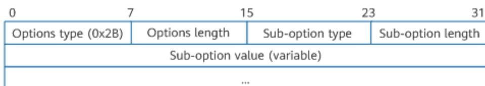
DHCPv4 servers and clients use Option 43 to exchange vendor-specific information. When a DHCPv4 server receives a DHCPv4 request message with parameter 43 encapsulated in Option 55, it encapsulates Option 43 in a reply message and sends the message to the DHCPv4 client.
