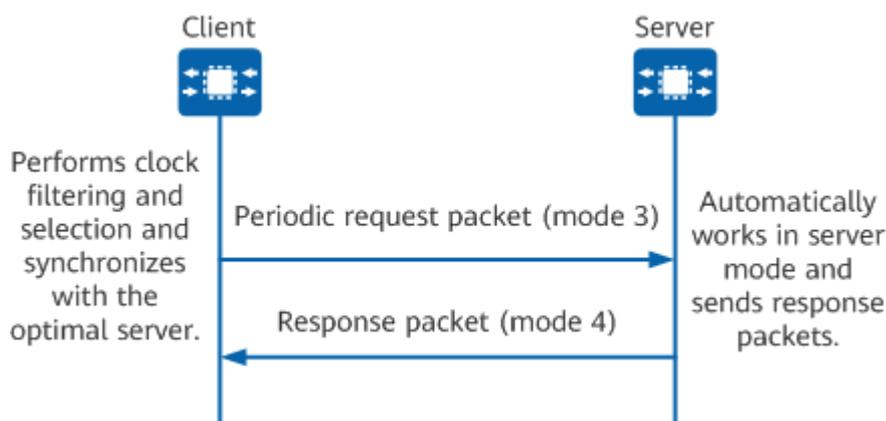
The packet exchange process in anycast mode is as follows:
