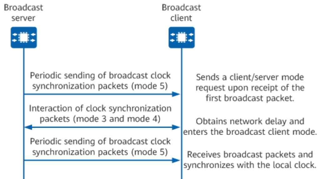
The packet exchange process in broadcast mode is as follows:
