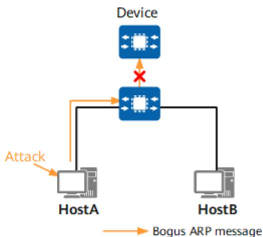
As shown in [Figure 7-22](#), HostA is attacked, and the attacker changes the source MAC address of an ARP request message sent by HostA. As a result, the source MAC address in the Data field of the message is different from that in the Ethernet header. If ARP message validity check is not configured, both HostB and Device learn the fake address information carried in HostA's ARP request message.
