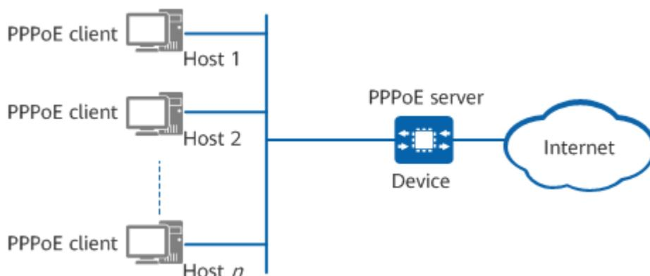
The PPPoE client at the peer end of a PPPoE server can be a host that has the dial-up software installed or a router.
