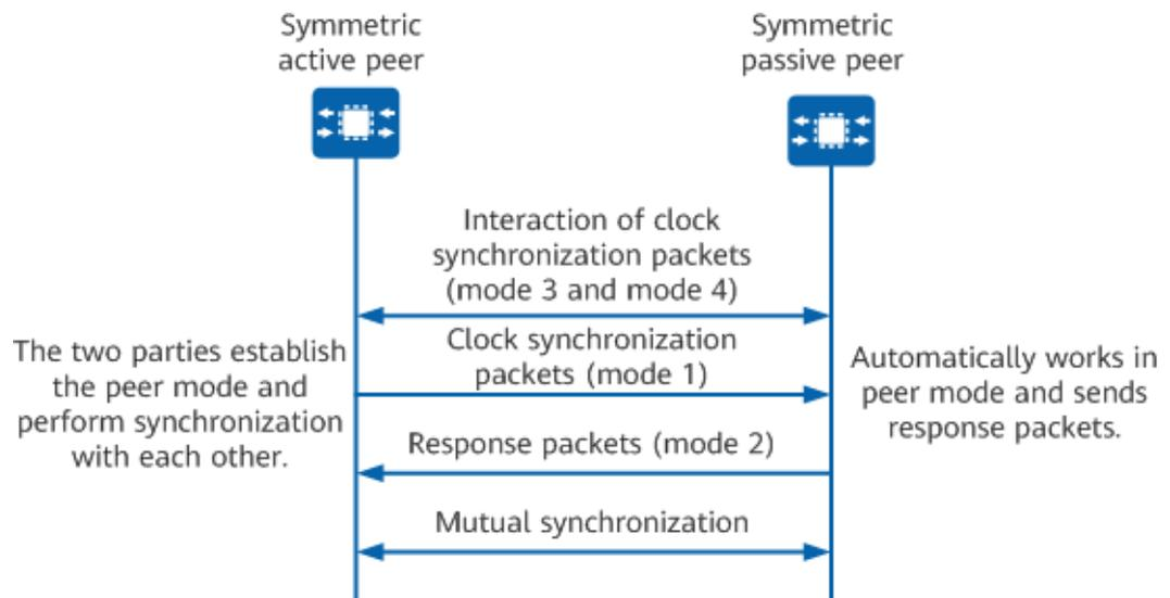
The packet exchange process in peer mode is as follows:
