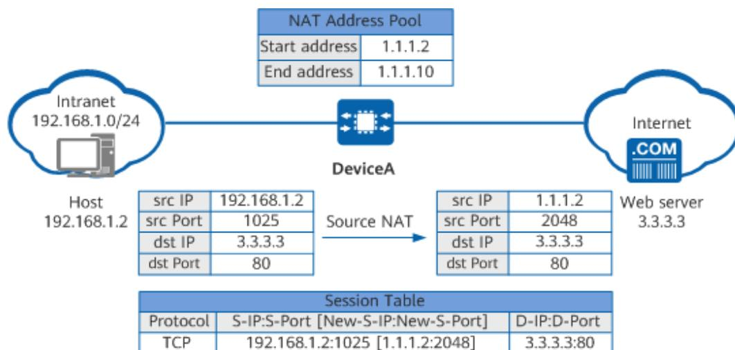
When a host on the intranet accesses the web server on the Internet, the NAPT process on DeviceA is as follows:
