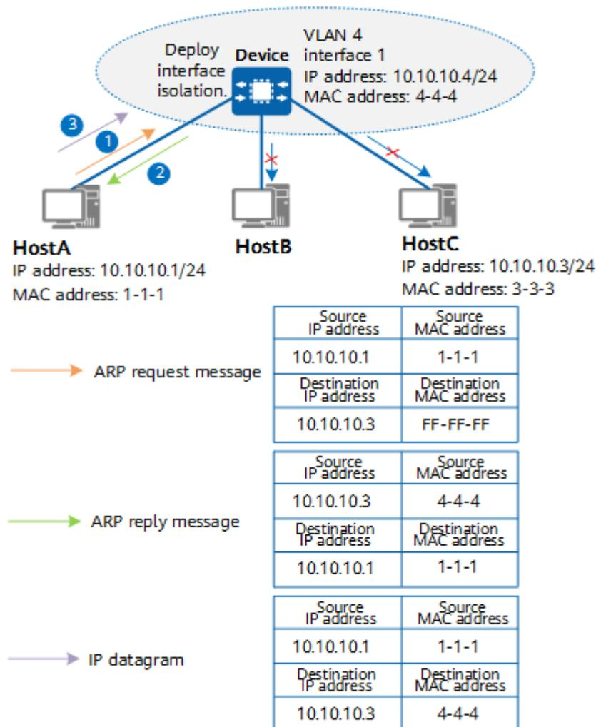
HostA, HostB, and HostC belong to the same VLAN, but HostA and HostC cannot communicate at Layer 2 because interface isolation is enabled on Device. To allow HostA and HostC to communicate, configure interface 1 on Device and enable intra-VLAN proxy ARP.
