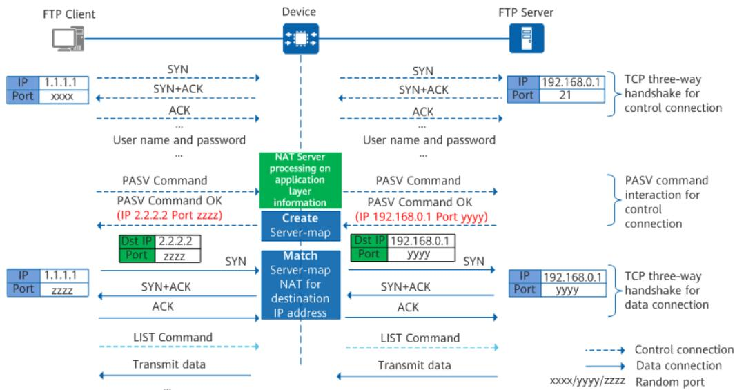
Before ALG is configured, the device translates only the IP address and port information in the packet header when performing destination NAT. However, the IP address and port information carried in the packet payload remain unchanged. If the IP addresses and port numbers of both sides are different, FTP cannot work properly.
