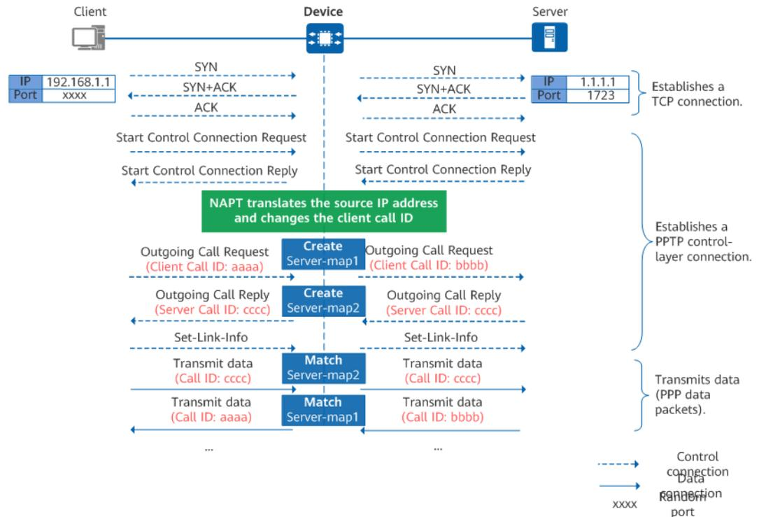
1. The client and the server establish a TCP connection through three-way handshake. A control connection session is generated on the Device. The IP address of the client is translated from 192.168.1.1 to 1.1.1.2 through source NAT, and the port is translated from **xxxx** to **yyyy**.
