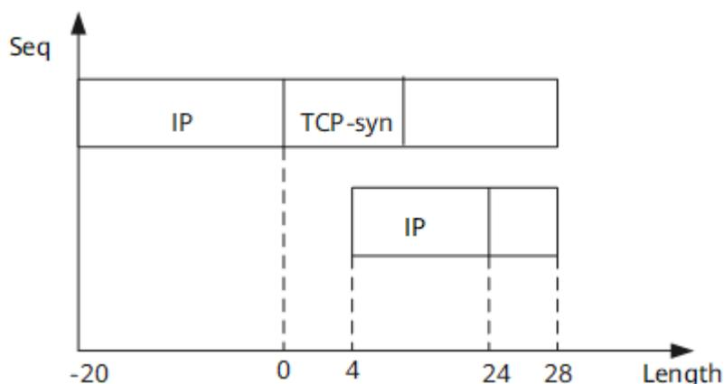
Syndrop attacks cause the system to restart or even crash. With defense against fragmentation attacks enabled, the device discards all fragments in a Syndrop attack.
