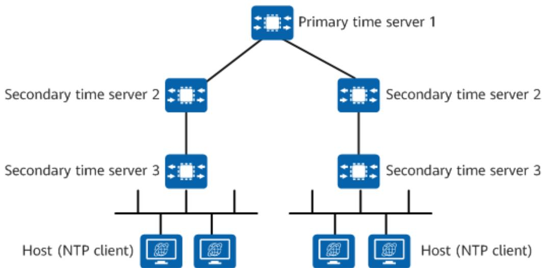
A primary time server is directly synchronized to a primary reference source, usually a radio clock or a global positioning system (GPS). A secondary time server derives synchronization through a primary time server or other secondary time servers, and uses NTP to transmit time information to other hosts on a local area network (LAN).
