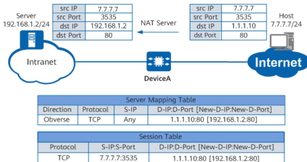
After NAT Server is configured on the device to determine the mappings between public and private IP addresses, the device generates server mapping entries to store the mappings. The entries will always exist unless the NAT Server configuration is deleted.
