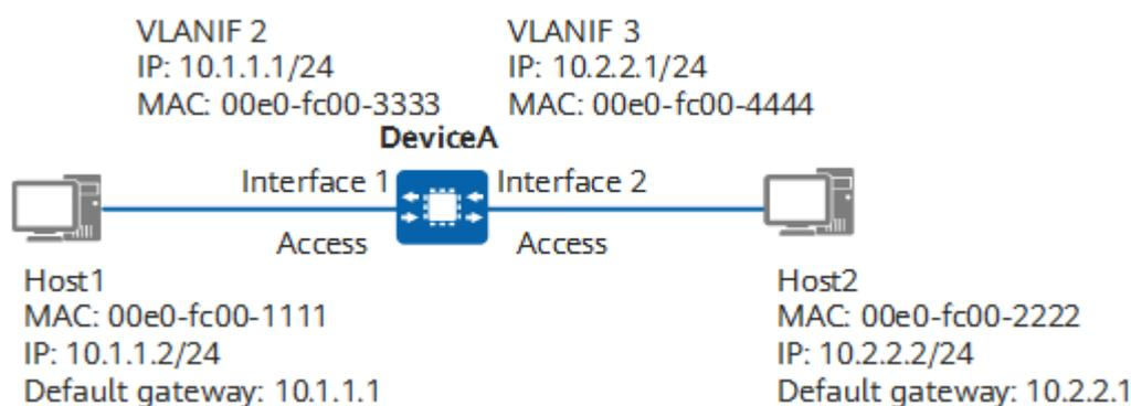
When Host1 sends a packet to Host2, the packet is transmitted as follows (assuming that no forwarding entry is created on DeviceA):
