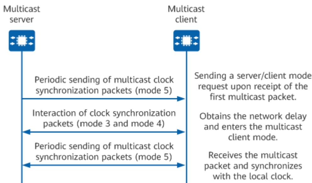
The packet exchange process in multicast mode is as follows:
