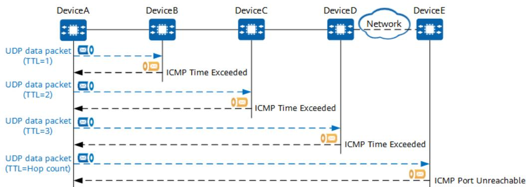
If no response packet is received within a specified period after a UDP packet is sent, a timeout prompt is displayed on the source. If a timeout prompt is displayed
