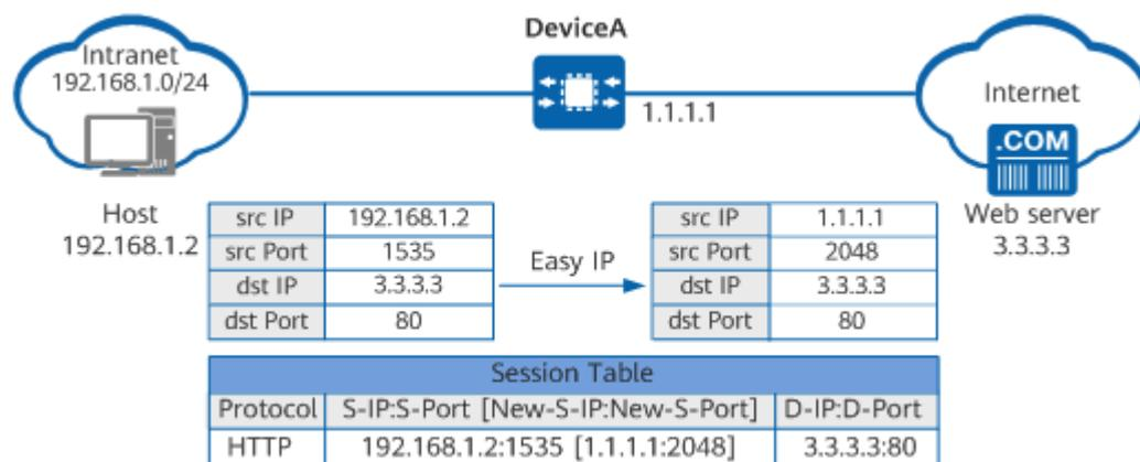
When a host on the intranet accesses the web server on the Internet, the Easy IP process on DeviceA is as follows:
