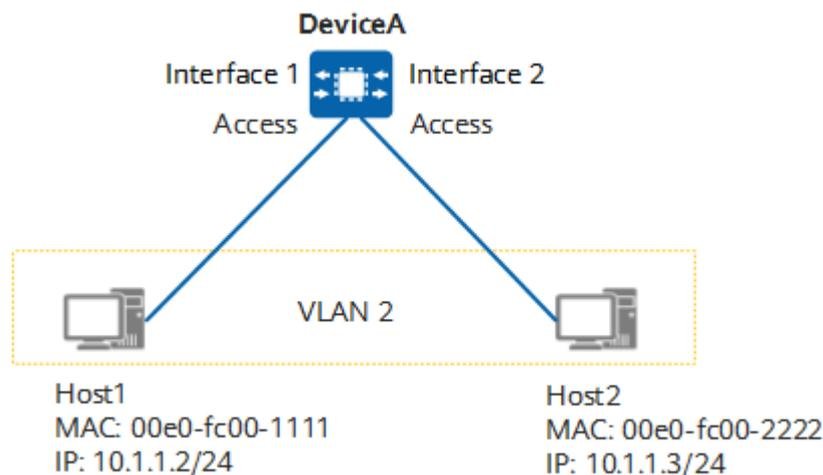
When Host1 sends a packet to Host2, the packet is transmitted as follows (assuming that no forwarding entry is created on DeviceA):
