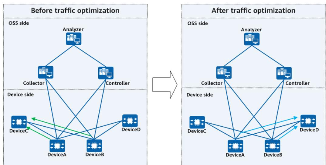
Compared with traditional network monitoring modes, telemetry greatly reduces both the adjustment and feedback delays. It frees you from being affected by traffic path changes and facilitates management and maintenance.
