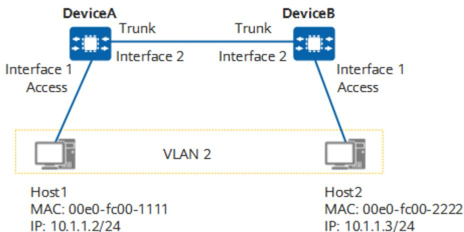
When Host1 sends a packet to Host2, the packet is transmitted as follows (assuming that no forwarding entry is created on DeviceA and DeviceB):
