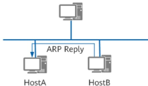
HostB compares its IP address with the destination IP address in the ARP request message. If the two addresses are the same, HostB adds the IP and MAC addresses of the sender (HostA) to the local ARP table. HostB then unicasts an ARP reply message, which contains its MAC address, to HostA, as shown in [Figure 7-17](#).
