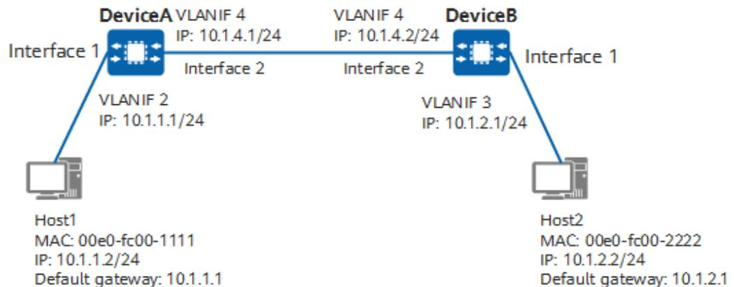
When Host1 sends a packet to Host2, the packet is transmitted as follows (assuming that no forwarding entry is created on DeviceA and DeviceB):
