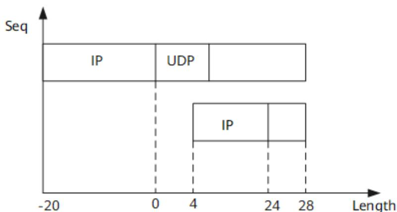
NewTear attacks cause the system to restart or even crash. With defense against fragmentation attacks enabled, the device discards all fragments in a NewTear attack.
