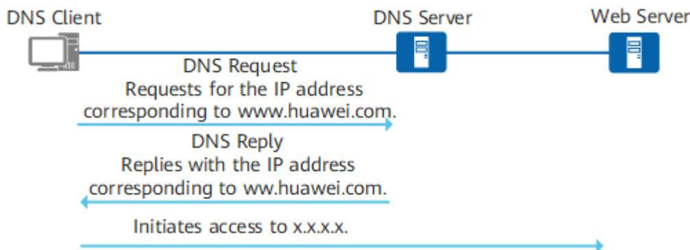
1. The client requests the IP address corresponding to the domain name **www.huawei.com** from the DNS server.
