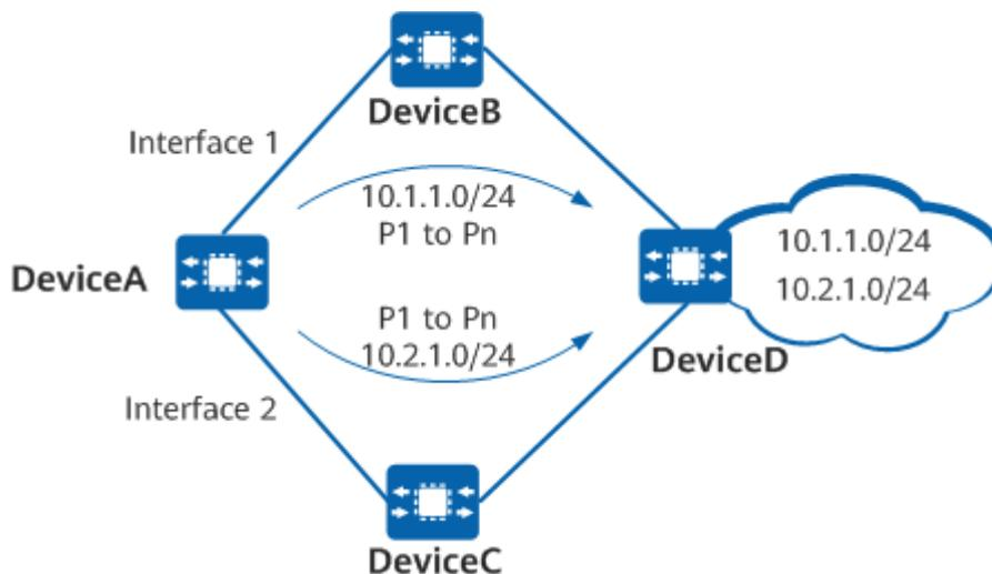
DeviceA has forwarded the first packet P1 to 10.1.1.0/24 through interface 1 and needs to forward subsequent packets to 10.1.1.0/24 and 10.2.1.0/24. The forwarding process is as follows:
