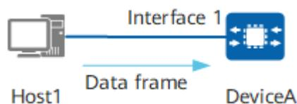
In **Figure 5-2**, Host1 sends a data frame to DeviceA. When receiving the data frame, DeviceA obtains the source MAC address (Host1's MAC address) and VLAN ID of the frame.
