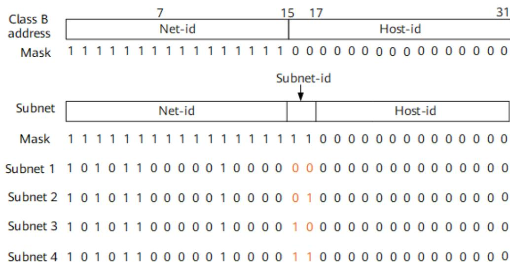
[Table 7-5](#) lists the network addresses (with the all-0 host ID), broadcast addresses (with the all-1 host ID), and host addresses of the preceding four subnets.
