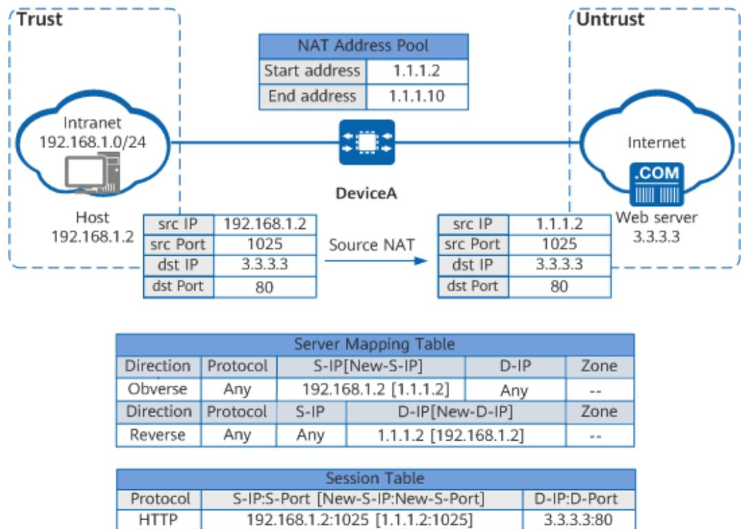
When a host on the intranet accesses the web server on the Internet, the NAT No-PAT process on DeviceA is as follows:
