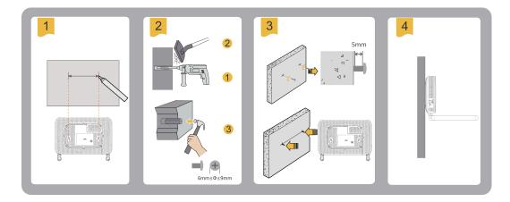
It is recommended that the screw be about 4 mm in diameter and longer than 20 mm. The screw head should be between 6 mm and 9 mm in diameter.
