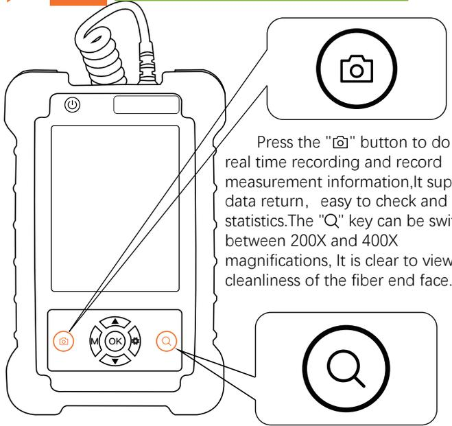
Press the "📷" button to do the real time recording and record measurement information, It supports data return, easy to check and statistics. The "Q" key can be switched between 200X and 400X magnifications, It is clear to view cleanliness of the fiber end face.
